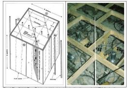
Fig. 1 The ONWUTerraTek heated block test for testing the coupled HTM (hydro-thermomechanical) behaviour of a jointed crystalline rock. Mean jointing trends are shown. A range of strain and deformation gauges are seen. (Hardin et al. 1981, Barton, 1982).
